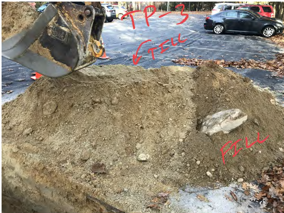
Photo 6: Stockpile of soil excavated from test pit HA21-TP3, consisting of light-brown Glacial Till to the left and medium-brown Fill to the right side of the of the stockpile. Cobbles and boulders are visible within the Glacial soils.
