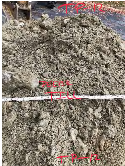
Photo 21: Stockpile of Glacial Till excavated from the bottom of test pit HA21-TP12.
