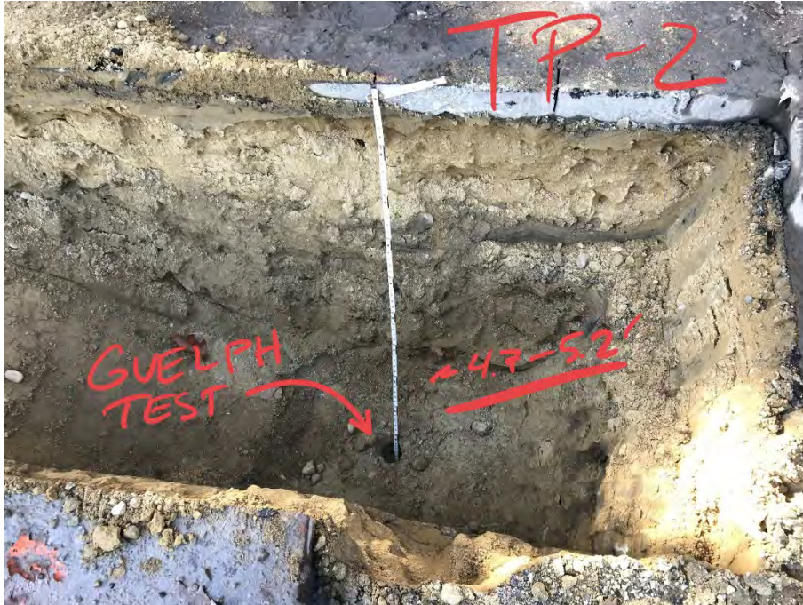
Photo 5: Guelph permeameter test performed in test pit HA21-TP2 from a depth of 4.7 ft to 5.2 ft bgs.
