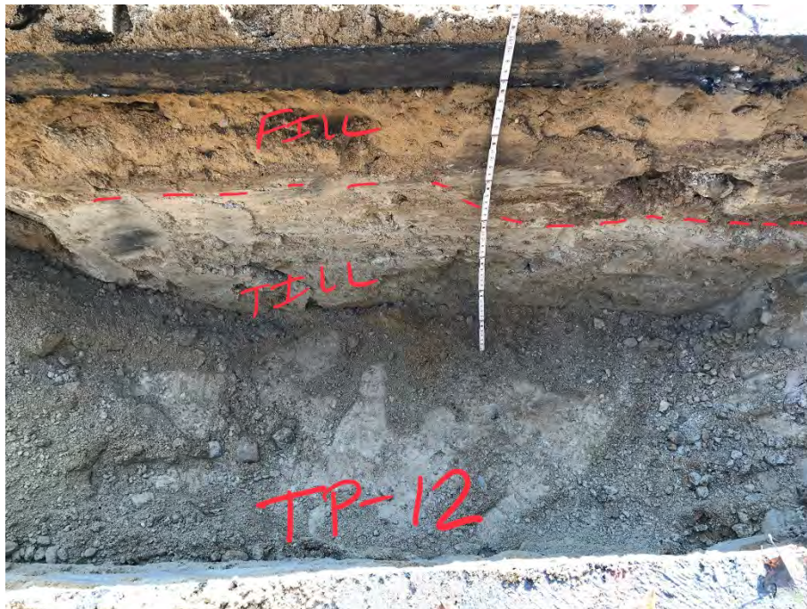
Photo 20: Fill overlying Glacial Till observed in the sidewall of test pit HA21-TP12.
