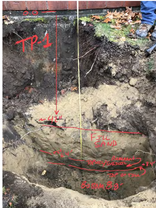
Photo 1: Sidewall at test pit HA21-TP1. Top of Glacial Till observed at approximately 8.4 ft below ground surface (bgs).
