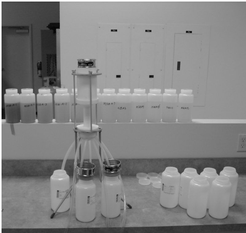
Figure 9 Side view of cone splitter apparatus prior to sample splitting using sieves
