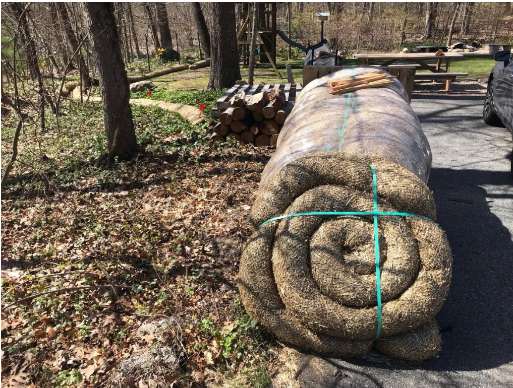
Picture 3. Straw wattles rolled up for future use for a landscaping project on the property of a single-family home in Andover.
