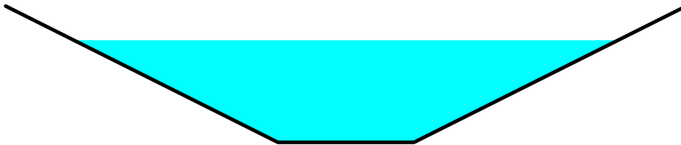
Reach 10R: Water Treatment Swale
