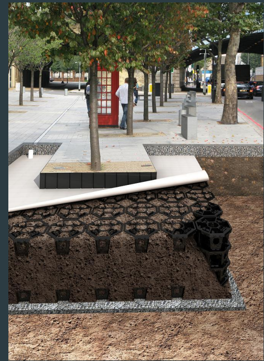
Underground Structural Cells
