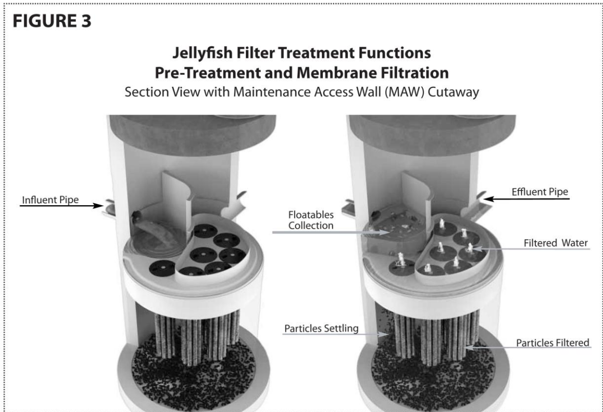
Figure 3 Jellyfish Filter Treatment Functions
