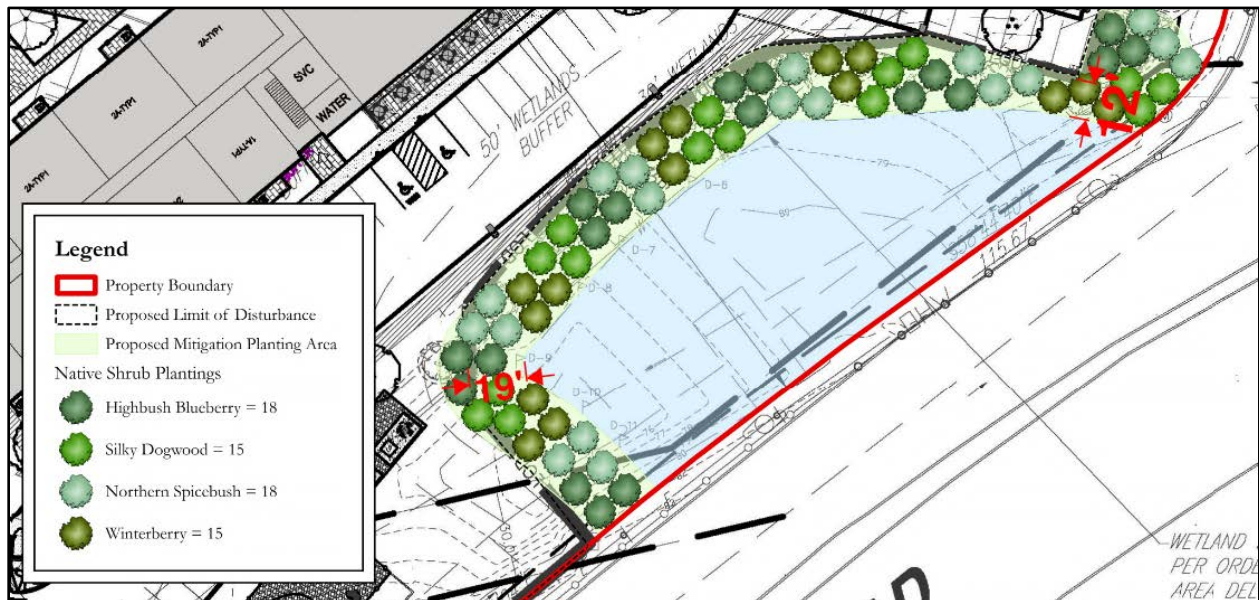
Figure 2. Screenshot of proposed Buffer Zone Mitigation Planting Plan with approximate measurements showing the width of the mitigation area in red
