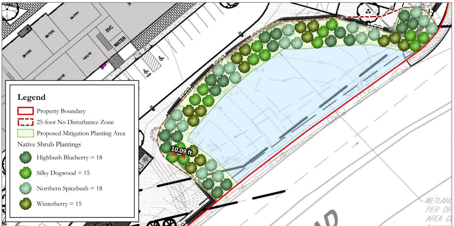
Figure 6. View of attachment Figure 3 of the revised ISMP prepared by Goddard Consulting. Note the 10-foot-on-center spacing of the proposed shrub planting based on the 1" = 40' scale.
